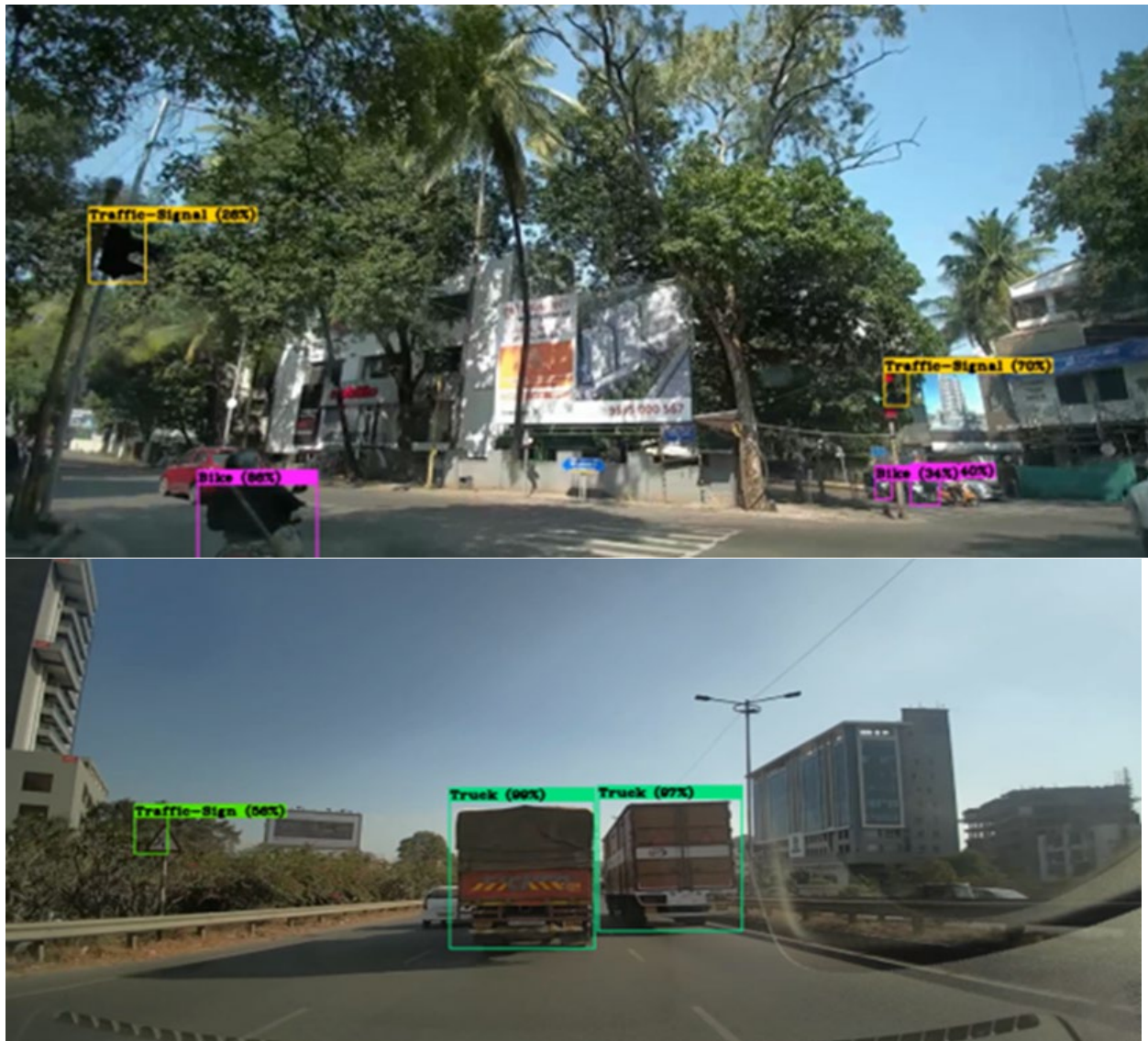
Figure 24. Traffic sign detection for Indian use case (detection of traffic signs, bikes and trucks as per Indian roads)
