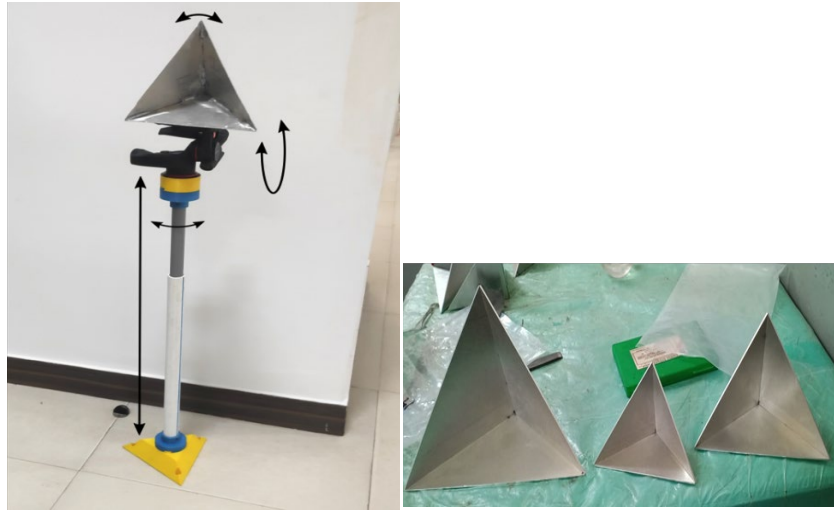
Figure 3. Radar Optimized Corner Cube Reflectors placed behind the rear of the vehicle
